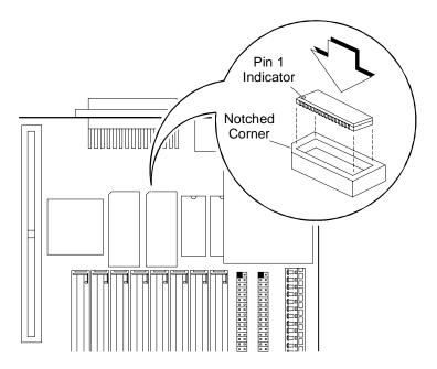
2. Gently insert a video chip into each of the upgrade sockets. Make sure that the pin 1 indicator on the chip matches the notched corner of the socket.
